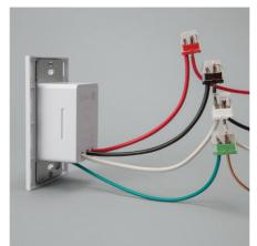
5 Connect Tapt assembly wiring with included push-in wire connectors. A push-in wire connector works as a 'finger trap' for wires; simply push wires into an available pole to lock. Connect as follows:
