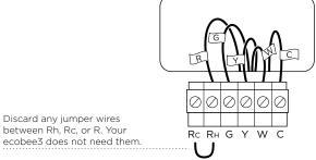
3. If you have used the wire label C, please skip step 3 and proceed directly to step 4. If you have NOT used the wire label C, proceed to Step 3: Install Power Extender Kit (PEK).
