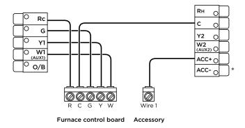
\*ecobee3 automatically connects Rc to ACC- when 1-wire configuration is selected during accessory setup.
