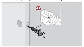
Reinstall the lock. If the turnpiece does not align with the torque blade, rotate the turnpiece 180° clockwise (you will need to use force when rotating the turnpiece, and you will hear it click).
