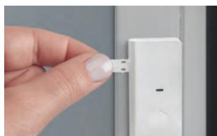
Remove the plastic tab that is sticking out from the battery portion of the sensor. This will activate the pairing mode. The LED light will flash green during pairing.
