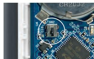
To reset or pair Tripper to a different Wink account or hub, open from the indent on the side of the main sensor. Press and hold the black tamper button while taking out the battery. Put the battery back in and let go of the tamper button.
